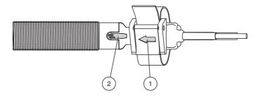
1. Attach the interface cable (1) to the rear of the sensor so that the marking arrow (1) points to the marking of the infrared interface (2) on the sensor.
